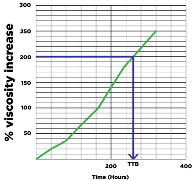
Fig. 8. Time To Break Vs. % Viscosity Increase. Wells, J. Novvi LLC, 2021
